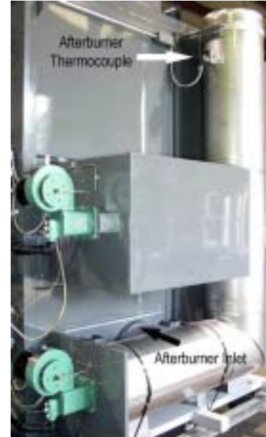
Figure 7 - Exterior primary and afterburner chambers are safe from damage. Notice that the afterburner controlling thermocouple is at the 1/2 second point relative to the inlet.
