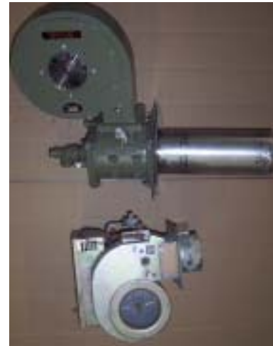
Figure 8 - Steelman's Hauck burners (top) compared to competitor's sheet metal burner.
